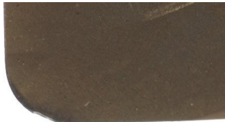
Tool wear after 30 hours of machining
