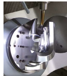
Small R corner finishing
