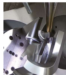
Small R corner finishing
