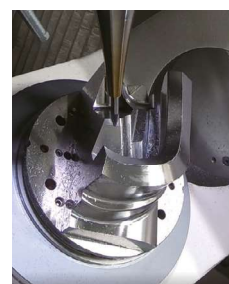
Inner curved wall finishing
