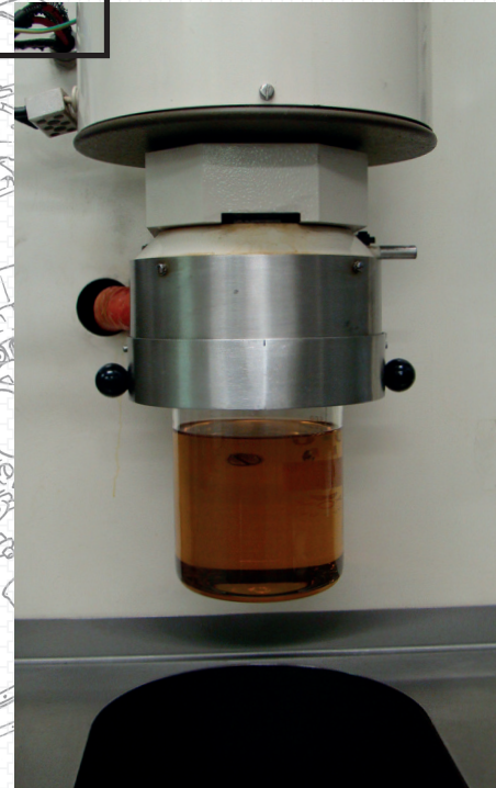
Drastimeter enabling to establish and check the characteristics of a quenching oil (drasticity).
